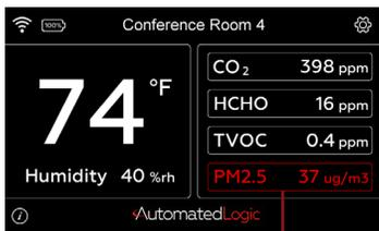
Clear visual indication of alarm conditions. Alarm thresholds are configurable to local compliance standards
