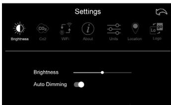
Configurable Brightness and Auto Dimming Settings
