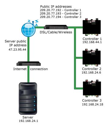
In this example, the controllers need to communicate with the WebCTRL® server and each other. The controllers are the only devices on the site's private network, or other devices present are benign. Each controller's BACnet firewall should allow BACnet communication with the WebCTRL® server's public IP address and with all private IP addresses so that the controllers can communicate with each other. The BACnet firewall prevents BACnet communication to the controller's public addresses.
