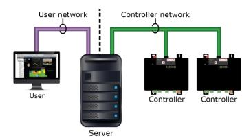
You can physically separate the user network and the BACnet network without any IP routing between them, or you can logically separate them at a switch using a Virtual Local Area Network (VLAN).
