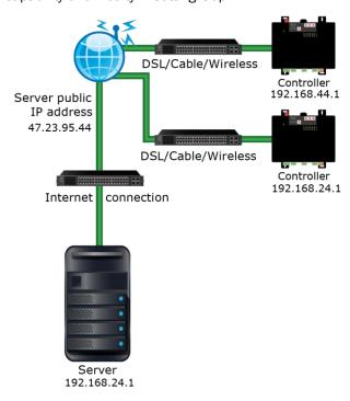
In this example, each controller needs to communicate with only the WebCTRL® server so their BACnet firewall's whitelist should have only the server's public IP address. The controllers do not need to communicate with each other.
