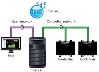
Do not permanently expose the WebCTRL® server or the BACnet network to the Internet. You can, however, allow users to access the WebCTRL® server through a secure VPN connection. If a NAT router or firewall is present on the LAN for other purposes, it should not have any ports forwarded to the WebCTRL® server or any controllers.
