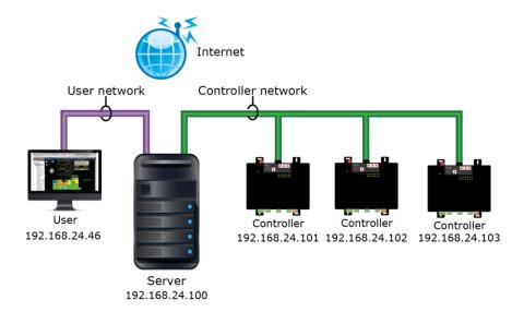
In this example, each controller's BACnet firewall should allow BACnet communication from the WebCTRL® server's IP address and the controller's IP addresses. The user at 192.168.24.46 should not be allowed BACnet communication with the controllers.
